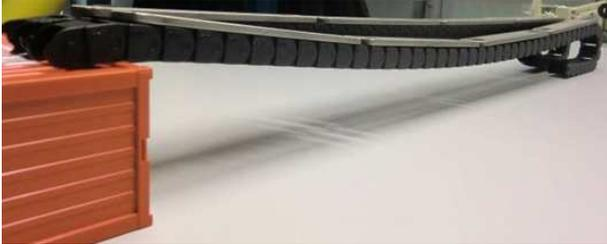
The E2.15 has a 23% higher unsupported length reaching the same sag as the 08 series, using the same load per meter.
